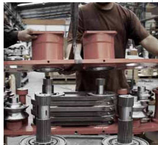
Two crawler units for driving the shutter motion
