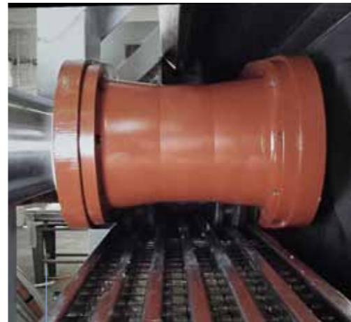
Crawler mechanism early unit on real scale test bench
