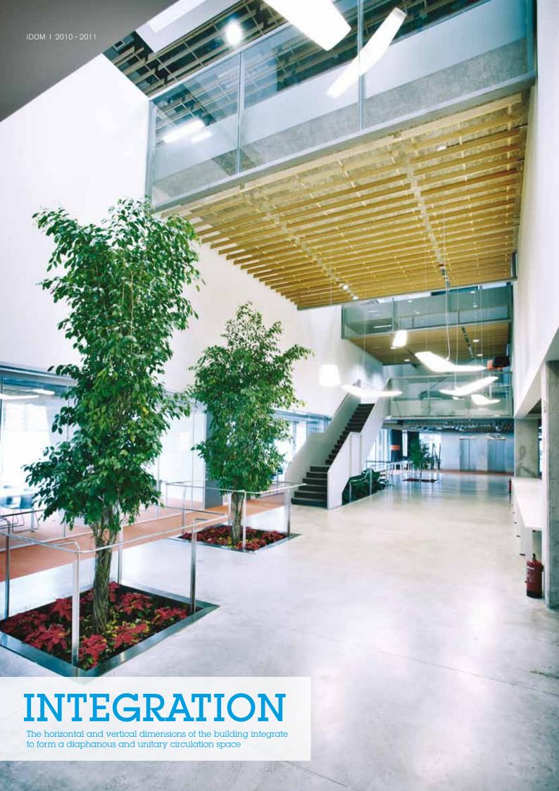
Natural ventilation is possible through connecting internal hallways, which cool the building without the use of the air conditioning system.
