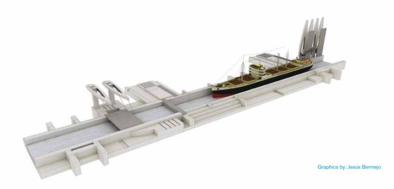
1.The new infrastructure, with 434 meters (1424 ft) long by 35 meters (115 ft) wide, allows the entrance of boats up to 292 meters (958 ft) long.
