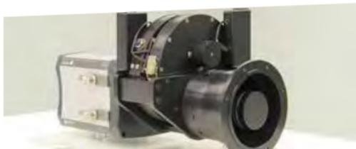
Wide FastCam is a wide-field imaging camera for the (TCS) conceived for obtaining extremely high temporal and spatial resolution images.
