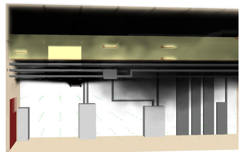
Fire spread and smoke along trays in a room of a NPP.
