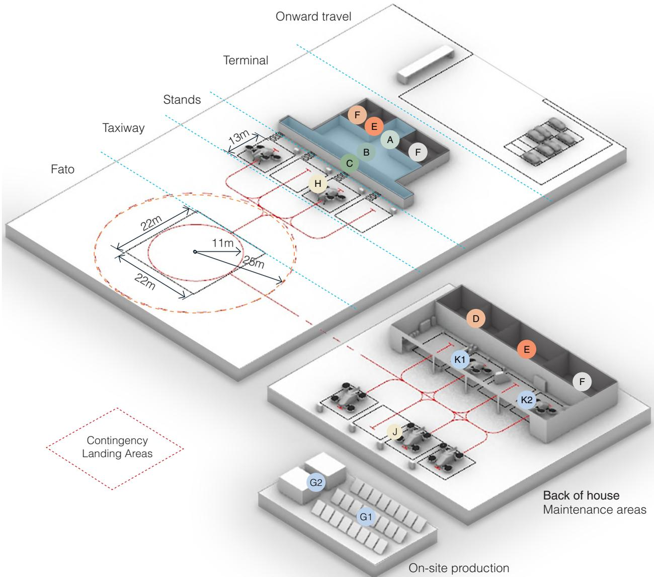
Adaptability, flexibility and simplicity. Vertiports can be easily assembled combining **pre-designed components as needed**, depending on the location and type of service. These are classified into three groups: Front-Of-House (FOH) areas, serving passengers; Back-Of-House (BOH) areas, serving the staff and the building; and Airfield, serving the eVTOL vehicles.
