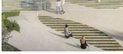
Mixed pavements for enhanced permeability
